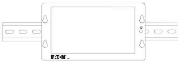
HMI display mounted on DIN rail, full length
